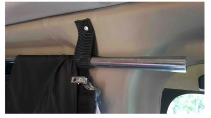
The **BALLISTIC CURTAIN** is easy to use. A curtain loop consists of a heavy duty 1.5-inch nylon strap and a screw. Install curtain loops on the cabin frame of the vehicle
